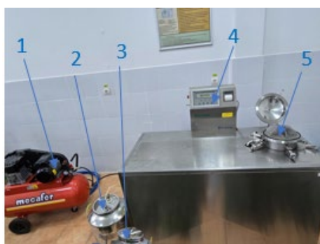
Figure 3.a. TIMATIC Duo percolator: 1 – compressor, 2 – expansion tank, 3 – extract collection vessel, 4 – control panel, 5 – extraction chamber
