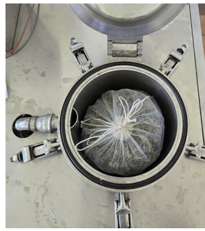
Figure 4.b. Placement of the permeable mesh bag with shredded lavender in the extraction chamber
