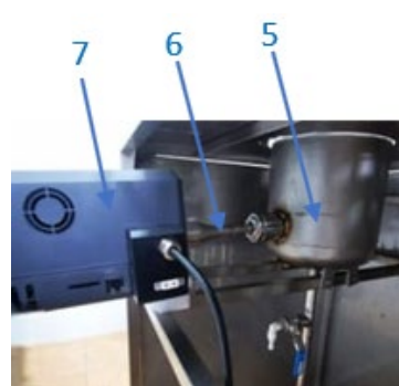
Figure 3.b. Configuration of the extraction chamber of the TIMATIC Duo percolator with the integrated Hielscher UP400St equipment: 5 – extraction chamber, 6 – sonotrode, 7 – ultrasonic generator
