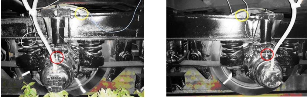
Fig. 8. Mounting accelerometers on the bogie frame and the axle-boxes.
