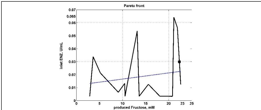
**Fig. 6.** The Pareto-optimal front in terms of Min. enzyme E consumption (initially added)-vs.- Max. P(D-fructose), for **OWL** limits (**Table 1**) of control variables. The marked SP is the same as the one chosen in **Fig. 4**. The blue line is the smoothed Pareto-optimal front.
