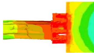
Fig.12. Temperature distribution during the continuous extrusion of simulation without control
