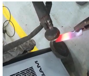
Fig. 3 Metal shrinking using induction heating
