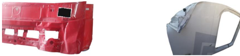
Fig. 1 Apparent damage that can be repaired by straightening
