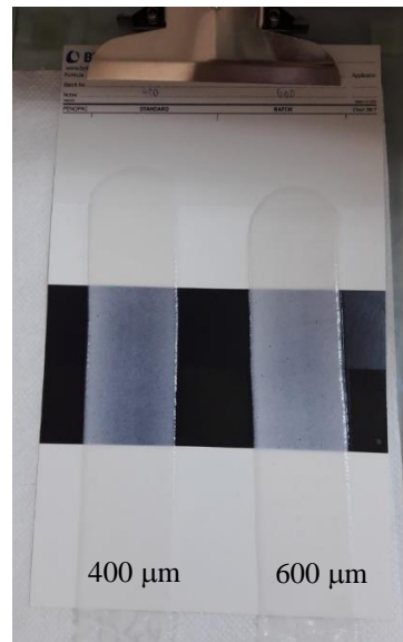
Fig. 7. Films with various thicknesses: a) coating with lower amount of AABSIP (paint 1); b) coating with a higher amount of AABSIP (paint 2)
