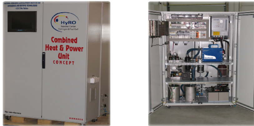
Fig. 2. Overview of the FCS-CHP system
