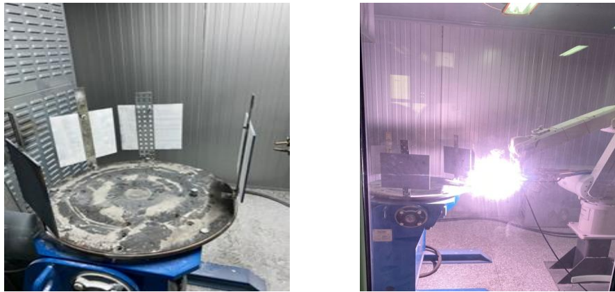
Fig. 1. The deposited tiles and the arm of the deposition installation
