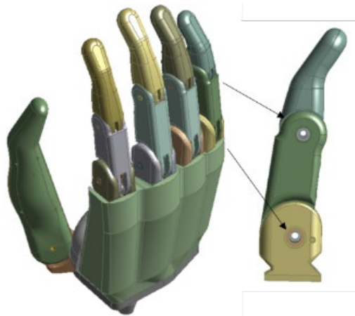
Fig. 7. Geometry simplification and revolute joint configuration
