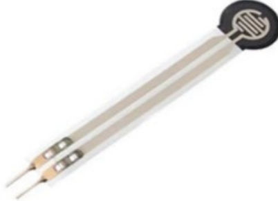
Figure 19. FSR402 resistive sensor
