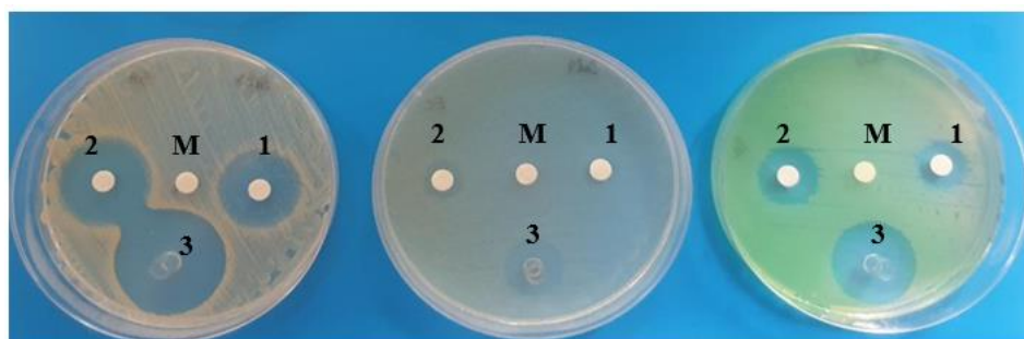
Fig. 7 Testing the antimicrobial activity of S4 by contact with Staphylococcus aureus (left), Escherichia coli (center), Pseudomonas aeruginosa (right) - 24 h reading to determine the presence of the inhibition zone around the samples
