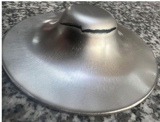
Fig. 26. Typical crack position on the real completely pressed component
