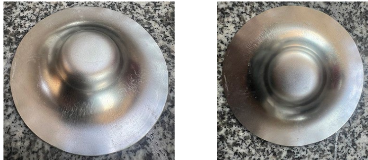
Fig. 10. Final shape of a good quality component made from martensitic steel (face and back)
