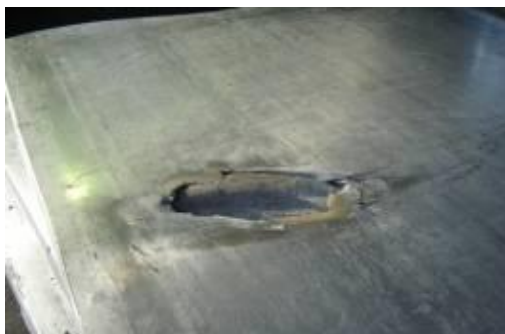
Fig. 6. Cracks appeared on the first two laminate
