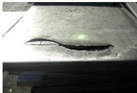
Fig. 6. Cracks appeared on the first two laminate
