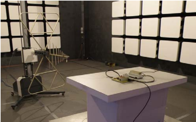
Fig. 7. View of the electronic module being tested for radiated emissions in a semi-anechoic chamber
