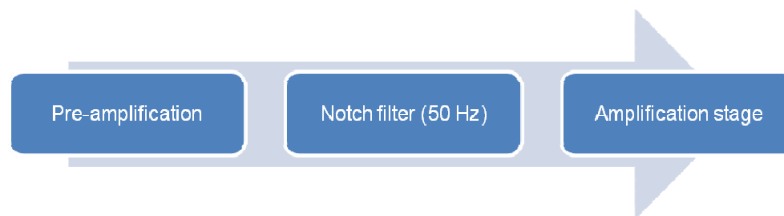
Fig. 1 Typical stages for a recording channel
