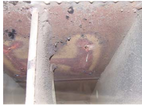
b) cracks on upper plate of bolster (view inside bolster)
