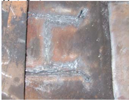
a) cracks on upper plate of bolster (view outside bolster)
