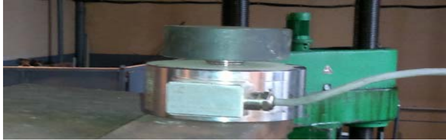
Fig. 8. Force cell HBM C2 200kN
