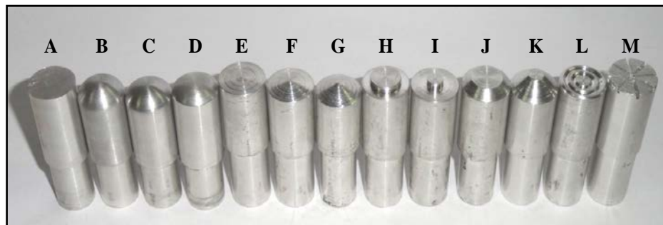
Fig. 3. Types of pre-surface used in inertia friction welding process
