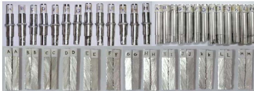
Fig. 7. A photograph of specimens after IFW process, initially and after the flash was removed
