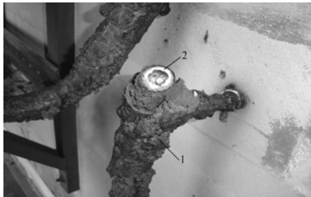
Fig. 11. Section through the cable presented in Fig. 4, after the thermal ageing at 400 °C for 2 hours: 1 – Sibralit A; 2 - XLPE insulation
