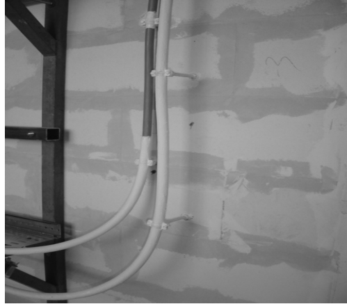
Fig. 10. Cable segment fixed in clams for 400 °C tests (the light grey area is covered with Sibralit A)
