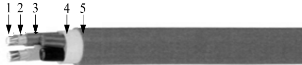
Fig. 6. Cable structure for motor alimentation: 1 – copper conductor; 2 – mica band; 3 – XLPE insulation; 4 – fireproof halogen-free filler; 5 – thermoplastic halogen-free jacket
