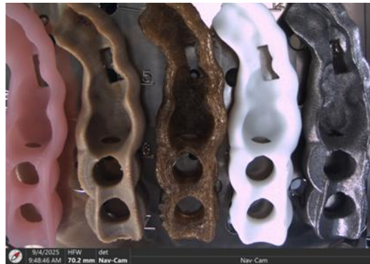
Fig. 2. 3D-printed dental guides for Scanning Electron Microscopy (SEM) analysis.
