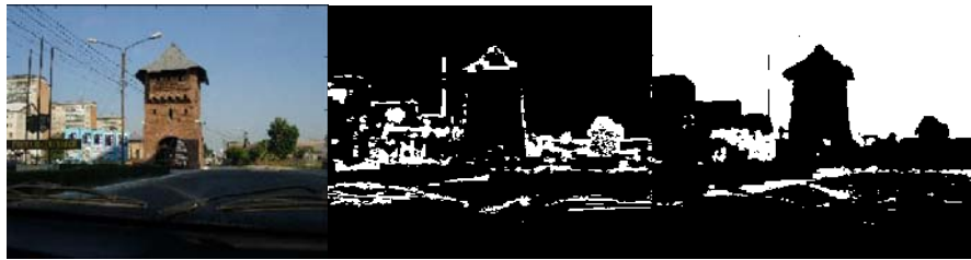
Fig. 5. Original image, green pixels (false colored in white), blue pixels (false colored in white). Green and blue pixels are 50% of image content. The edge orientation distribution is not that uniform, thus the image does not fit in the “landscape” class. The distance with respect to the landscape class boundary is very small; the problem comes from the estimation of edge direction for edges located in areas darker than the lower luminance threshold used for color estimation. These edges (which may be wrong) contribute in the particular case of this image to the non-uniformity of the edge direction distribution.
