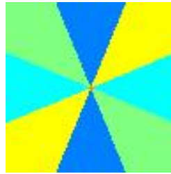
Fig. 1. LUT orientation table storing vertical, horizontal and diagonal orientation codes according to vertical and horizontal gradient magnitudes
