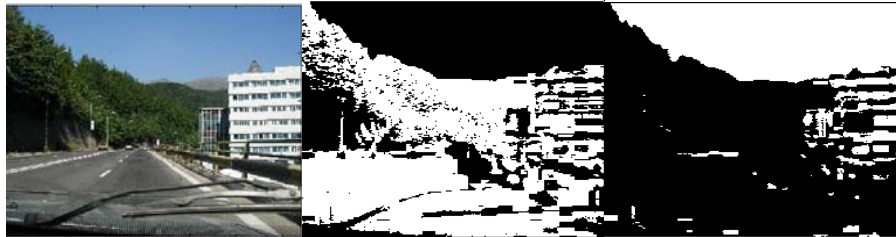
Fig. 6: Original image, green pixels (false colored in white), blue pixels (false colored in white). Green and blue pixels are 75% of image content. Edges have a uniform orientation distribution, thus the image fits in the “landscape” class.
