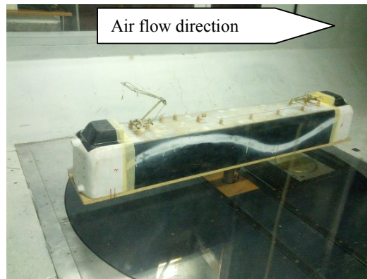
Fig. 10. Test no 6 – LE 5100kW with from the front pantograph high, meaning of air flow at the maximum working height, articulation arms towards the inside of locomotive and air conditioning on box
