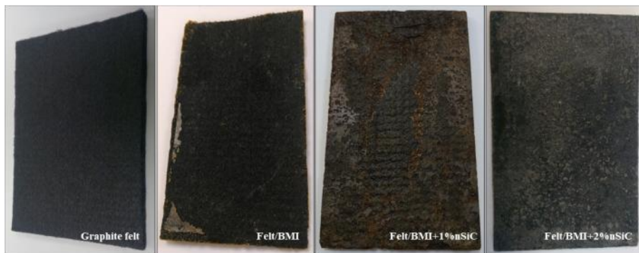
Fig. 2. Composites with high thermal protection (Felt/BMI/nSiC)
