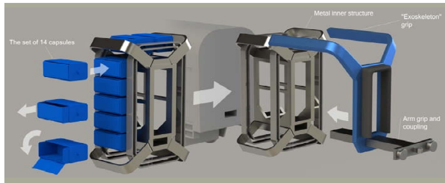
Fig. 9 Internal structure of the dynamic module
