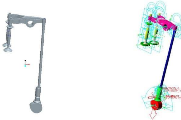
Fig.4. Three-dimensional model of valve train Fig.5. Multi-body dynamics model for valve train
