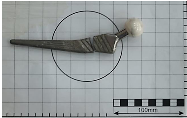
Fig. 3. General view of failed HIP prosthesis
