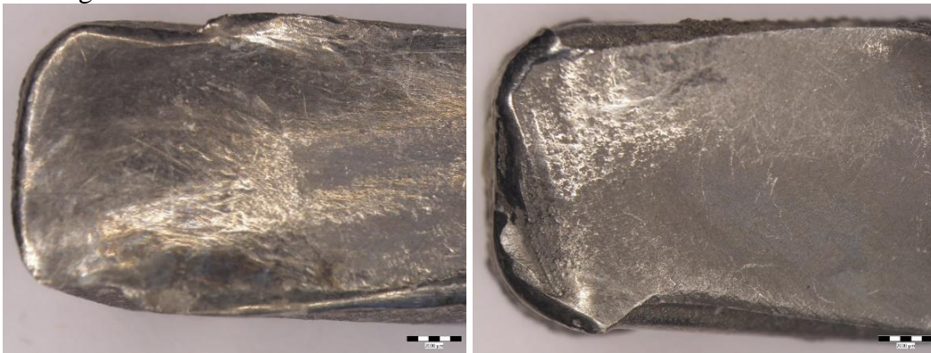
Fig.4. Macrostructural appearance of different marginal areas of the intramedullary stem of the explanted hip prosthesis
