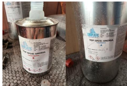
Fig 1 The resin and the hardener used in the manufacture of brake cylinders are currently used by the manufacturer
