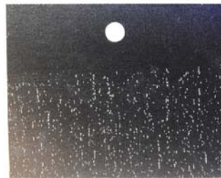
Fig. 2: Specimen SS301 after anodic polarisation showing pits
