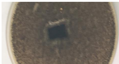
Fig. 2. Exposure of paint samples on CZAPEK-DOX „B” medium (P4 without UV exposure – pure culture of Aspergillus niger – 28 incubation days).
