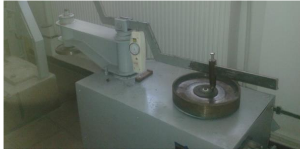
Fig.4. Laboratory stand used for the study of wear using the pin-on-disk method
