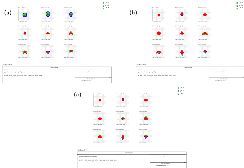
Fig.8 (a) (b) and (c) respectively represent the theoretical design point diagrams of the system at low temperature of -50^{\circ}\text{C} , normal temperature of 22^{\circ}\text{C} , and high temperature of 70^{\circ}\text{C}
