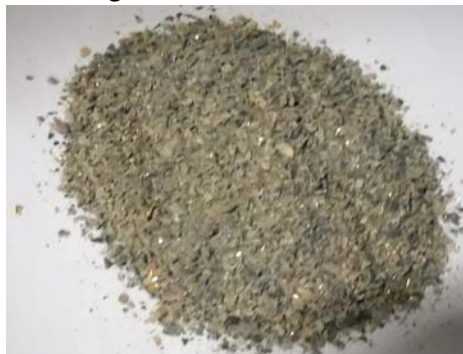
Fig. 4. Aspect of plastic microprocessors milled in the cutting knives mill
