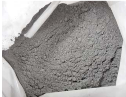
Fig. 5. Aspect of ceramic microprocessors milled in the oscillating disk mill
