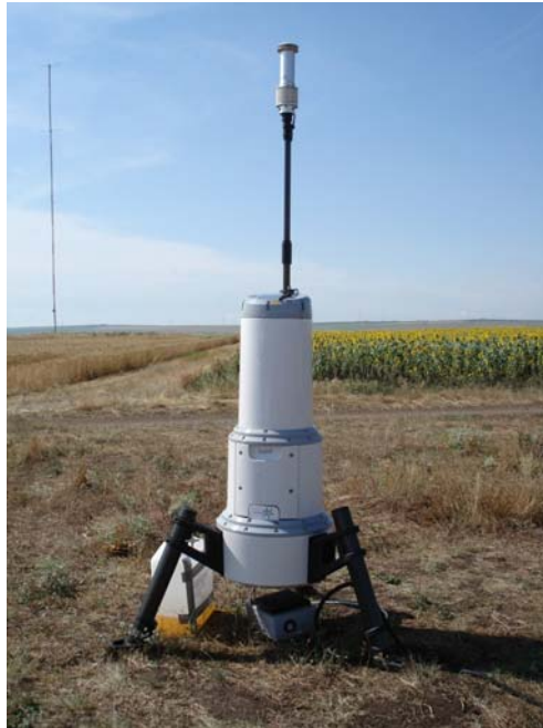
Fig. 2: The installed LIDAR at Mihai Viteazu with the 40 m mast in the background.
