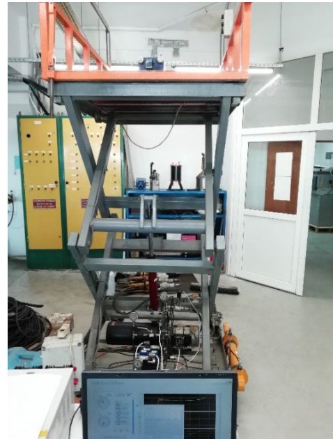
Fig. 2. Lifting platform with energy efficiency system - physical model
