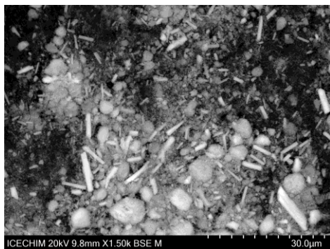
Fig. 9. SEM image of ZnHAP 1:1.
