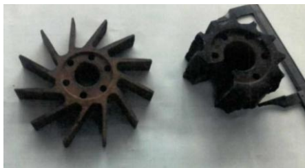
Fig..3 Pump rotors with broken blades
