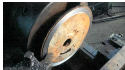
Fig..4 Disc discharge pump with surface wear
