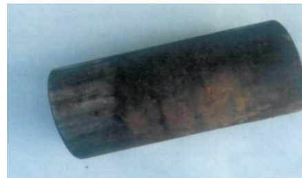
Fig..2- Brateş pump wear bush, corroded
