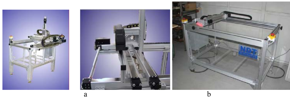
Fig. 3 Ultra PAC a – AUT motion system ; b. AUT system - Immersion tank.
