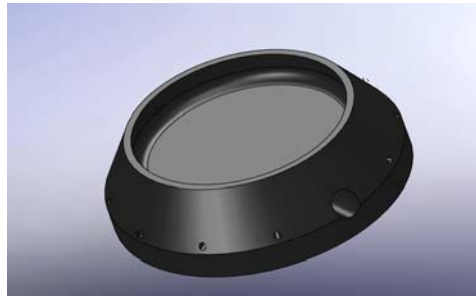
Fig. 3. Device for material heating during laser processing.
