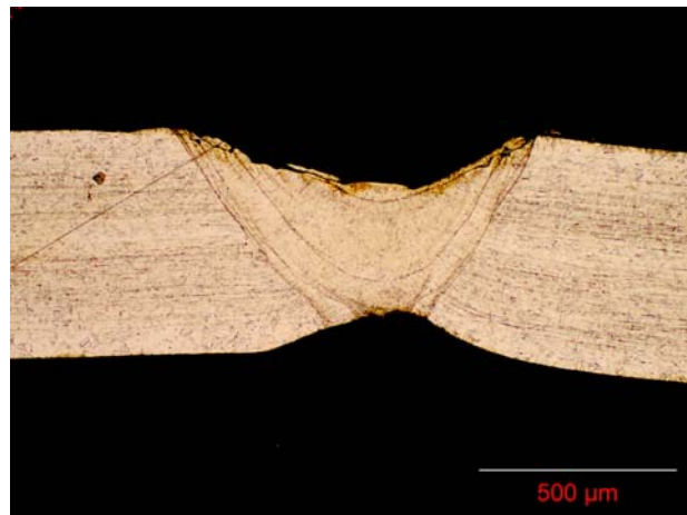
Fig. 8. Welded probe cross-section and dimensioning.
