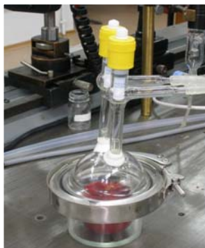
Fig. 2. The device used to contain fruits for the prelevation of the gas samples
