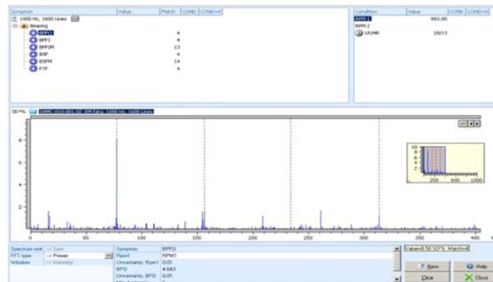
Fig. 2 b) The FFT analysis of the shock impulse signal
