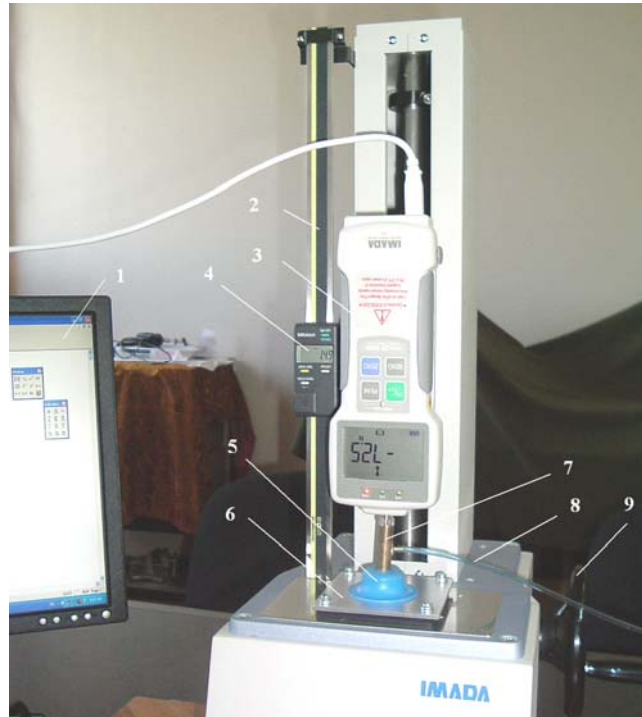
Fig. 6. Testing stand of IMADA used to determine the cup characteristic for normal force.
