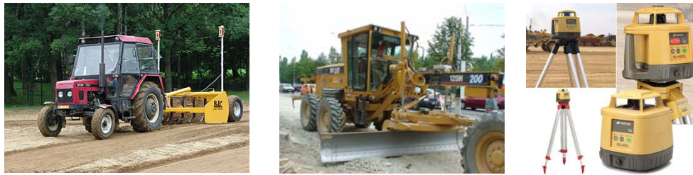
Fig. 3. Leveller and autograder equipped with laser controlled modular systems.
