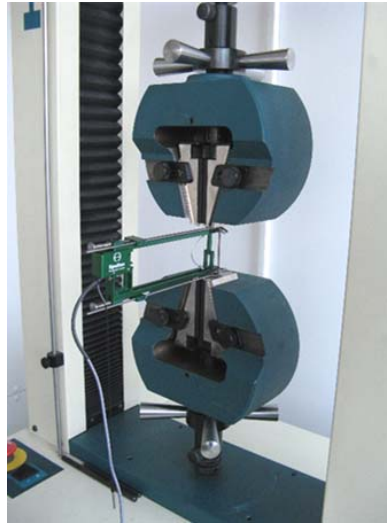
Fig. 2. Clamping the tests on the H10KT tensile tester
