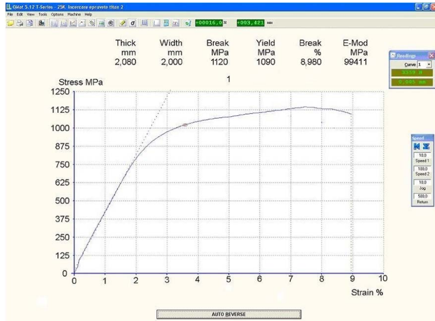
Fig. 2. Stress-strain curve of Ti-6Al-4V test sample no. 1
