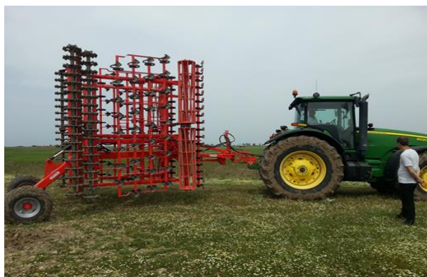
Fig. 5. Sandokan vibrocultivator in transport position
