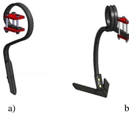
Fig.1. Vibratory tines mounted on elastic supports [14] a) Gamma type; b) Delta type
