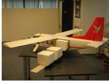
Fig 2. Scale mockup with internal blocks distribution for inertia simulation
