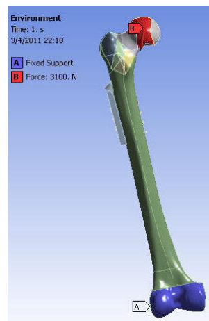
Fig. 3. Oblique load at the proximal end of the femur and total constraint (fixed support) at the distal end
