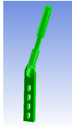
Fig. 2. External fixed implant with regular H orientation for normal rigidity
