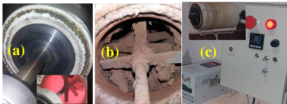
Fig. 1. The design of thermolysis equipment: (a) thermolysis chamber; (b) the thermolysis chamber inside view; (c) the induction heating unit of the coil
