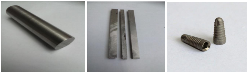
Fig.4. Technological steps for obtaining of the self-tapping screw dental implant [9]
