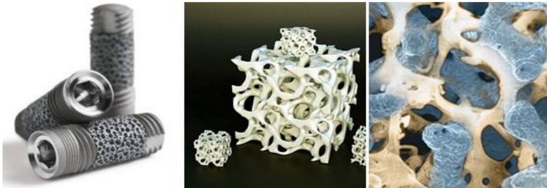
Fig.2. Trabecular metal implant that imitates bone architecture [14]
