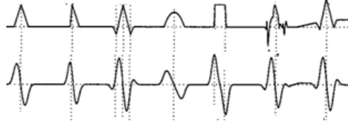
Fig. 2. The top figure shows waves of different shapes and the bottom figure shows the zero crossings of the dyadic wavelet transform DyWT for scale j = 3
