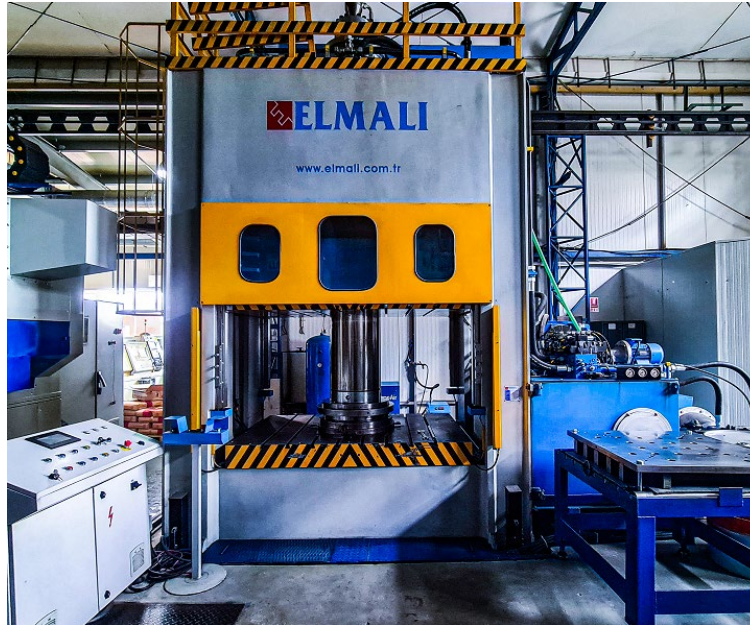
Fig. 1 Typical deep well press of 5MN with proportional servovalves [1]
