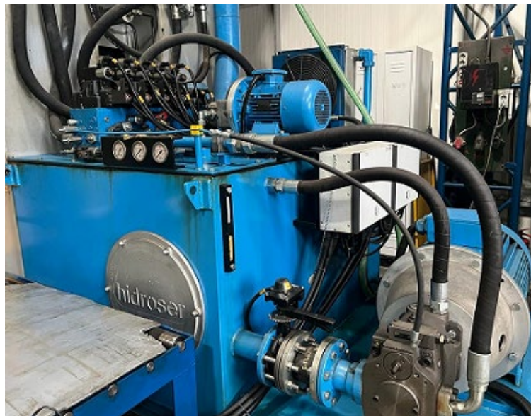
Fig. 2 The hydraulic oil supply system and the flows control section: the oil tank, the servopump Parker PV046R1, the Parker proportional servovalves block, and the auxiliary electropump [1]
