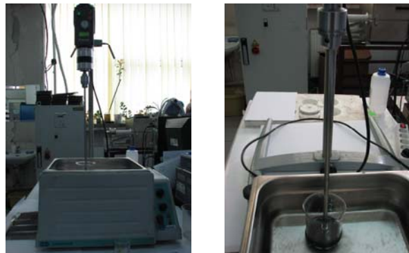
Fig. 1 Aspects during ultrasonic and mechanical treatment on the mixing composite material (metallic powder with resin and hardener)
