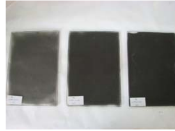
Fig. 13 Electromagnetic screens made from Fe with concentration of 4%, 10%, 16%
