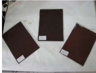
Fig. 12 Electromagnetic screens made from Cu powder with concentration of 4%, 8%, 16%
