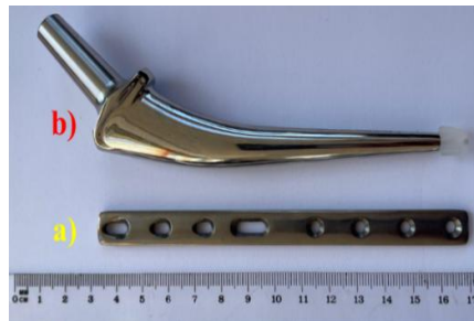
Fig. 2. Experimental orthopedic implants used in the study: a) plate for long bone fractures – sample S1, b) femoral stem hip prosthesis – sample S2
